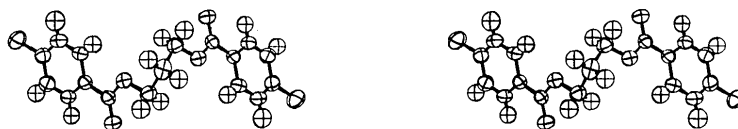
Fig. 1. A stereoscopic view of the structure of one molecule of trimethylene glycol di- p -chlorobenzoate. The twofold axis of rotation is vertical.
